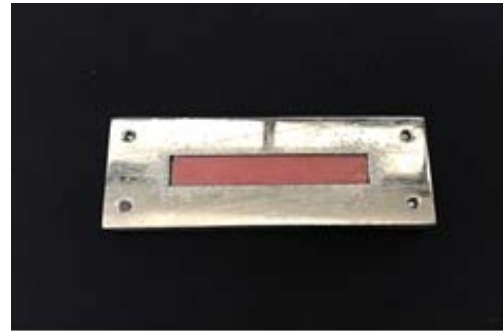
Figure 2. Metal mold recommended by ISO 20795-1
