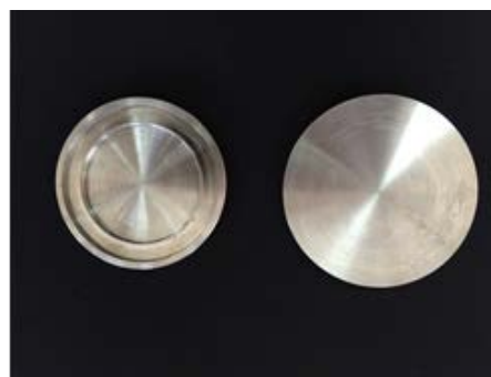
Figure 1. Metal mold recommended by ISO 20795-1
