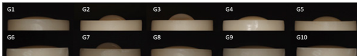
Figure 1 Contact angle of deionized water on etched and unetched lithium disilicate disks treated with different types of silane coupling agent. Group without hydrofluoric etching: (G1) Control, (G2) Kerr silane primer, (G3) Monobond N, (G4) RelyX ceramic primer, (G5) Experimental silane primer. Group with hydrofluoric etching prior to silane application: (G6) HF-no silane, (G7) HF-Kerr silane primer, (G8) HF-Monobond N, (G9) HF-RelyX ceramic primer, (G10) HF-Experimental silane
